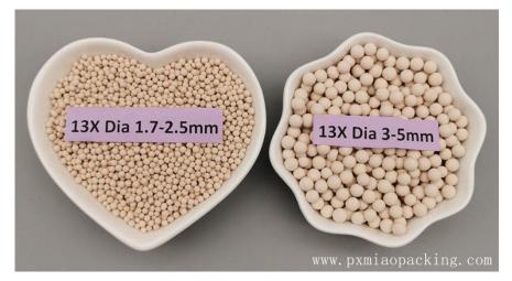
Molecular Sieve 13X is the sodium form of the type X crystal and has a much larger pore opening than the type A crystals. The pore size 13X molecular sieve is about 10 Å . It can absorb any molecular smaller than 10 Å , mainly used as catalyze carrier, co-absorption of CO2 and H2O, H2O and H2S, as desiccant for medical and air compressor system, and can also be adjusted to fit other various applications.
