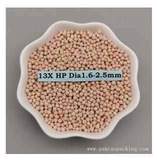
Molecular Sieve HP is mainly used in PSA oxygen concentrator and oxygen concentrator device, and as well as the industrial PSA unit, with the characteristics of higher  $N_2$  adsorption capacity and  $N_2$  with  $O_2$  selectivity, easy desorption and etc.
