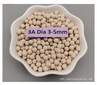
The pore size of 3A molecular sieve is 3 Å. It does not adsorb any molecular larger than 3 Å. It is an alkali metal alumina-silicate, the potassium form of the typ A crystal structure. 3 Angstrom, is obtained when part of the sodium ions of the 4 Angstrom sieve are replaced by potassium ions. Will adsorb, in sequence of adsorption rate, helium, neon, nitrogen and water
